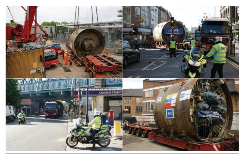
ALS subcontracted the use of a vessel bridge trailer to transport the 23t & 40t pieces and a modular 5 bed 5 trailer with a drawbar unit for the heavier pieces at 103t & 105t.
