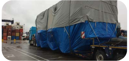
41T Genset Tank & 9.3T Lid on wafer deck trailer
